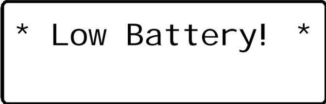
If *EDDI* is already awake and the battery level drops below a certain threshold, a flashing battery symbol will appear on the screen together with the current sensor readings.
