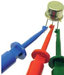
Fig. 5: The Active Component Analyser, the DCA55, uses three colour coded hook-on probes for testing (see text).
