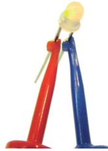
Fig. 4: The probes used on both units are of the wire-ended hook-on type. (See text for comments).
