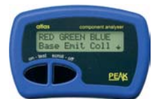
Fig. 2: The second unit to be reviewed is the Peak Component Analyser DCA55, which identifies and analyses active devices (see text).
